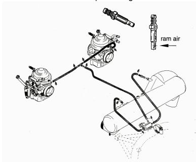
The standard routing of the float bowl vent is to inside the airbox. When the Enrichener Solenoid is activated the float bowl vents are routed to a ram air port near the turbo inlet tube.
