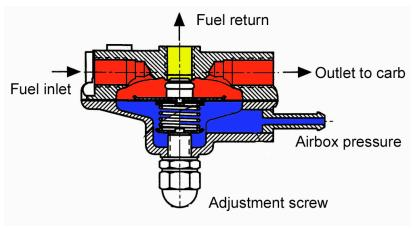
In the event that the fuel pressure gets too low, due to a maladjustment or malfunction of the fuel regulator, the engine would experience fuel starvation due to the higher airbox pressure sensed in the carburetor float bowls not allowing the fuel supply to enter. A high fuel pressure can result from regulator maladjustment, malfunction or restriction in return line. A properly adjusted fuel regulator will maintain fuel pressure above airbox pressure within the following parameters:
