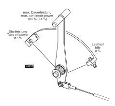
this position the TCU will add full boost as its logic thinks you are going to full power. From 108% to 110% throttle position it is very difficult to set your manifold pressure to a given value, as the throttle becomes very sensitive in this area. For this reason it is recommended to make a detent or mark on your throttle so the pilot can recognize exactly where 100% is, allowing the pilot to avoid the sensitive 108% throttle position.
