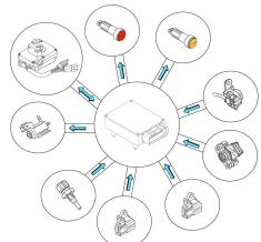
Two operating lights are required for the TCU, which are to be installed in the aircraft panel. As the master switch is turned on both lights are momentarily activated to indicating power is supplied to the TCU and that normal electrical power-up has occurred.
