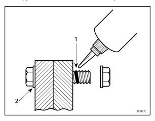
Figure 1.5: Application for uncovered holes (Bolts and nuts)
