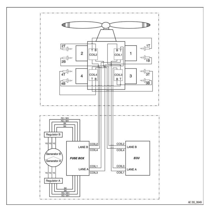
Figure 13.3: Layout plan allocation (cylinder/LANE)
