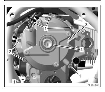
Figure 2.42: Ignition housing screw diagram
