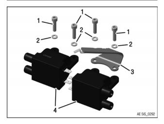
Figure 13.11: Double ignition coils
