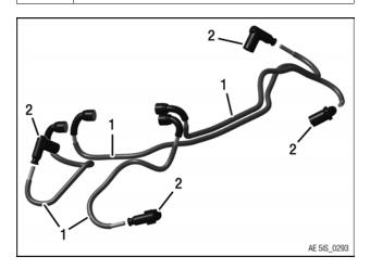
1 Spark plug connector 2 Ignition cable assy.
