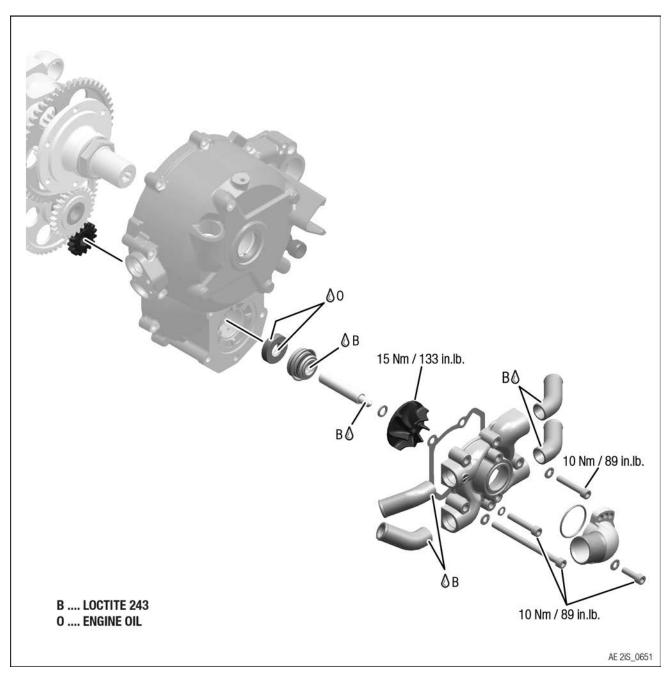
Figure 14.3: Cooling system
