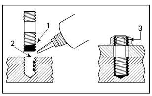
Figure 1.7: Application for stud installation in blind holes
