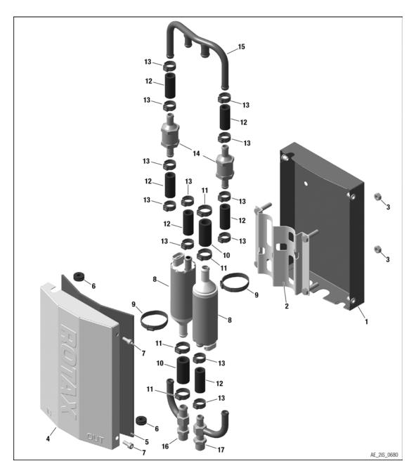
Figure 11.2: Fuel pump single parts
