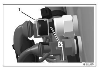
Figure 18.41: Position of the clamp
