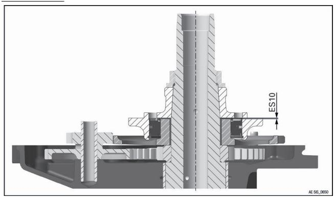
Figure 7.22: Free wheel gear
