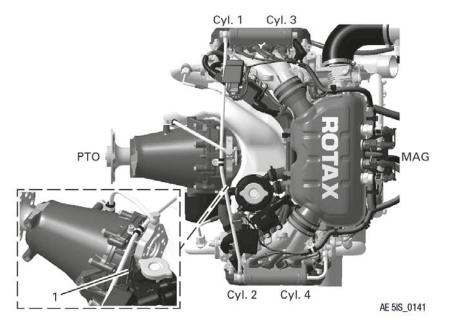
Figure 1.1: Engine serial number
