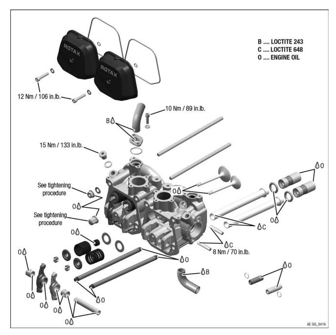
Figure 8.3: Cylinder head
