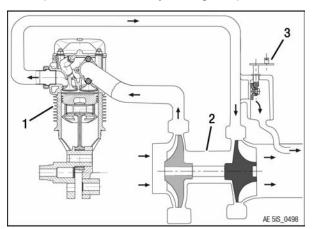
Figure 21.3: Schematic of a boost pressure
