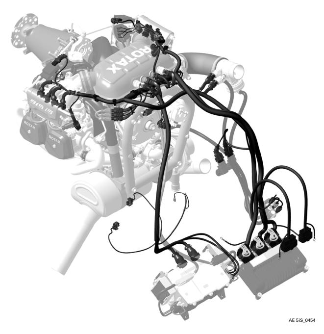
Figure 17.1: Wiring harness (main strand)
