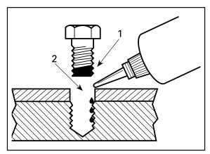
Figure 1.6: Application for blind holes
