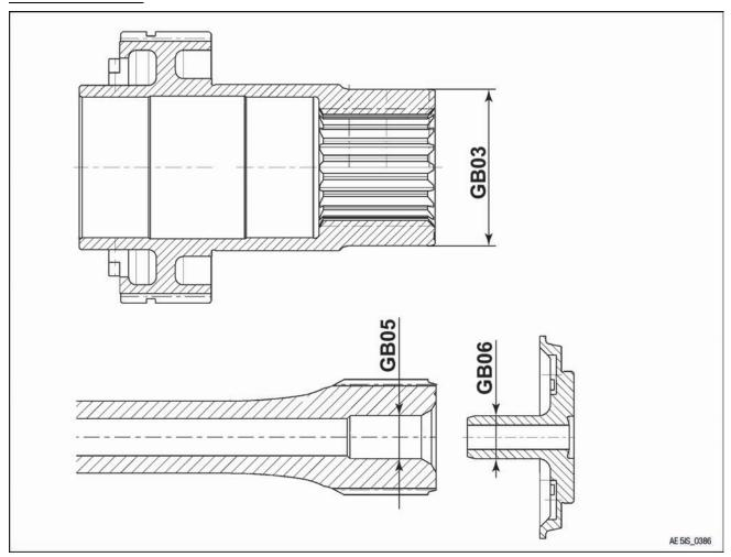
Figure 3.12: Intermediate shaft, Torsion shaft
