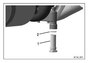
Figure 21.21: Plug screw assy.
