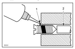
Figure 1.9: Application for an adjustment screw
