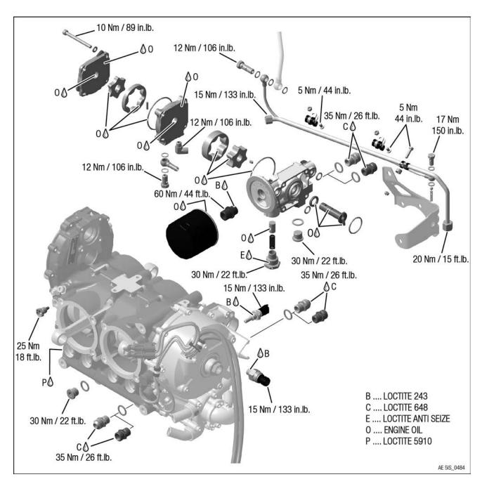
Figure 22.3: Lubrication system
