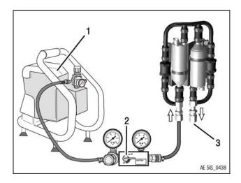
Figure 11.74: Leakage check
