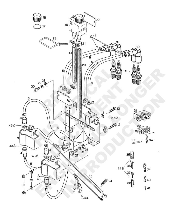
DELBEHAELTER, ZUENDSPULEN, TRAEGERPLATTE DIL TANK, IGNITION COILS, SUPPORTING PLATE
