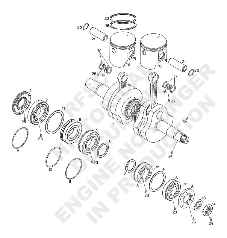
KURBELWELLE, KUGELLAGER, KOLBEN CRANKSHAFT, BEARINGS, PISTONS
