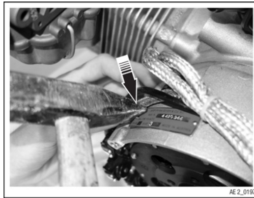
Figure 1.7: Installation of the engine type plate
