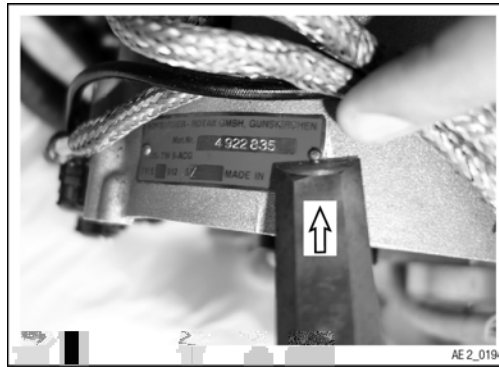
Figure 1.3: Remove of the grooved pin
