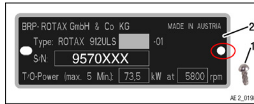
Figure 1.5: New engine type plate with pin
